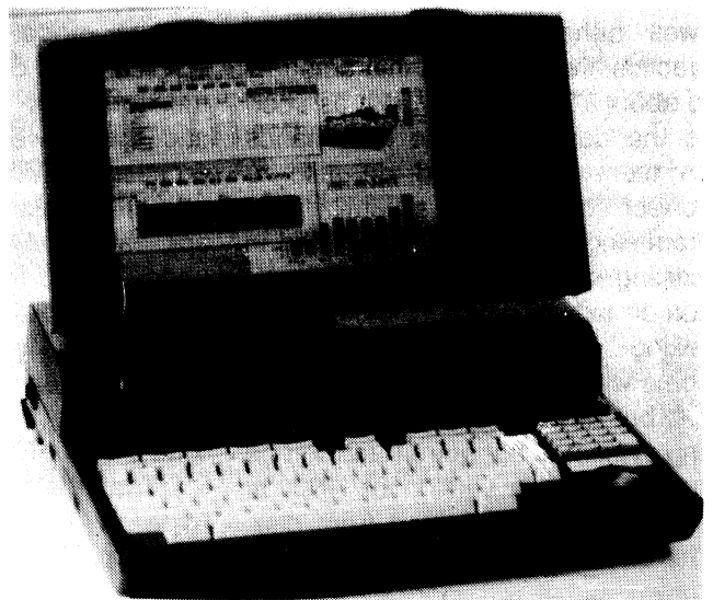
Stacy - The Stacy laptop computer is compatible with the thousands of 1040ST packages already on the market. The portable system includes 1 to 4 MB RAM and optional hard drives.
